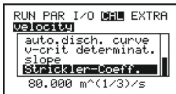
Fig. 25-9 Manning Strickler v-crit determination
