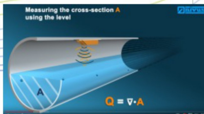
The flow measurement principle as video under: www.nivus.com
