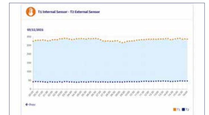
Thermal measurement: Temperature trend inside and outside the insulation
