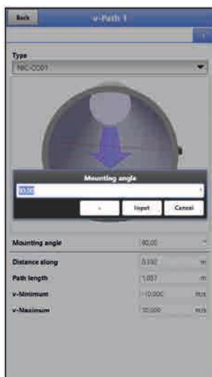
Fig. 33-4 Enter the mounting angle (Clamp-On)
