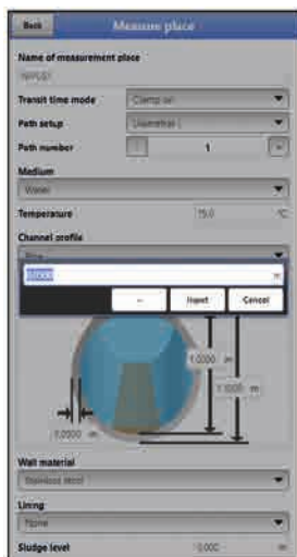
Fig. 33-2 Specifying pipe dimensions
